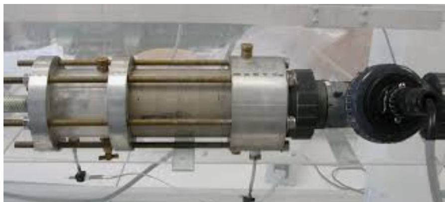
Figure 5 : Essai Pinhole test
