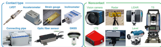
Figure 1: Sensors used for structural displacement measurement [12]
