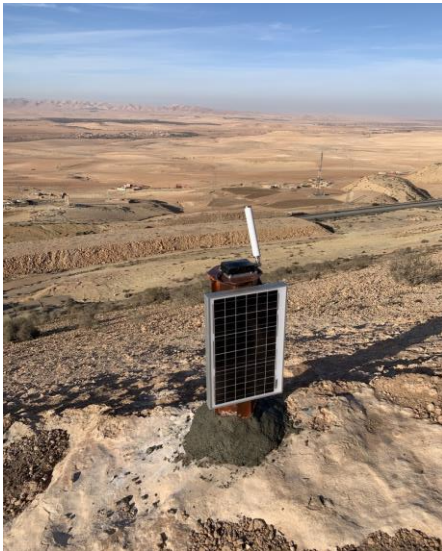
Photo 1. Examples of GPS sensor structures with autonomous solar panel power supply
