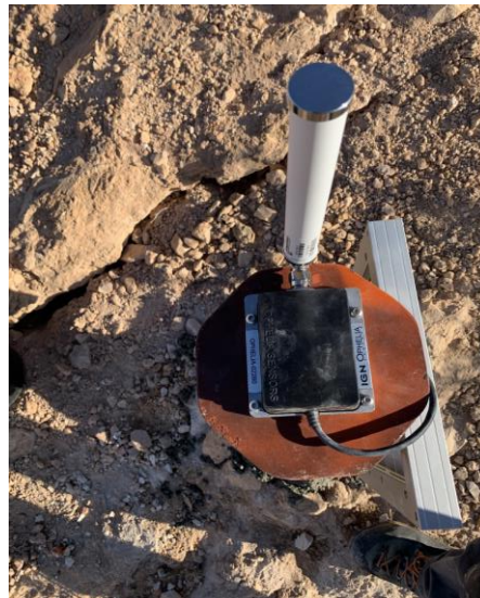
Photo 1. Examples of GPS sensor structures with autonomous solar panel power supply
