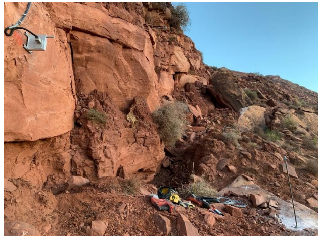
Photo 4. Fixed part on rock and mobile part on anchor bar
