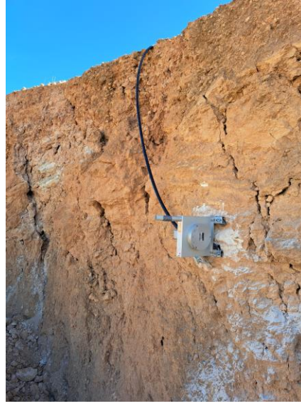
Photo 3. Cable extensometers for crack gap measurement
