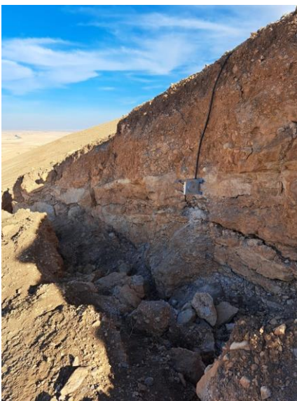
Photo 3. Cable extensometers for crack gap measurement
